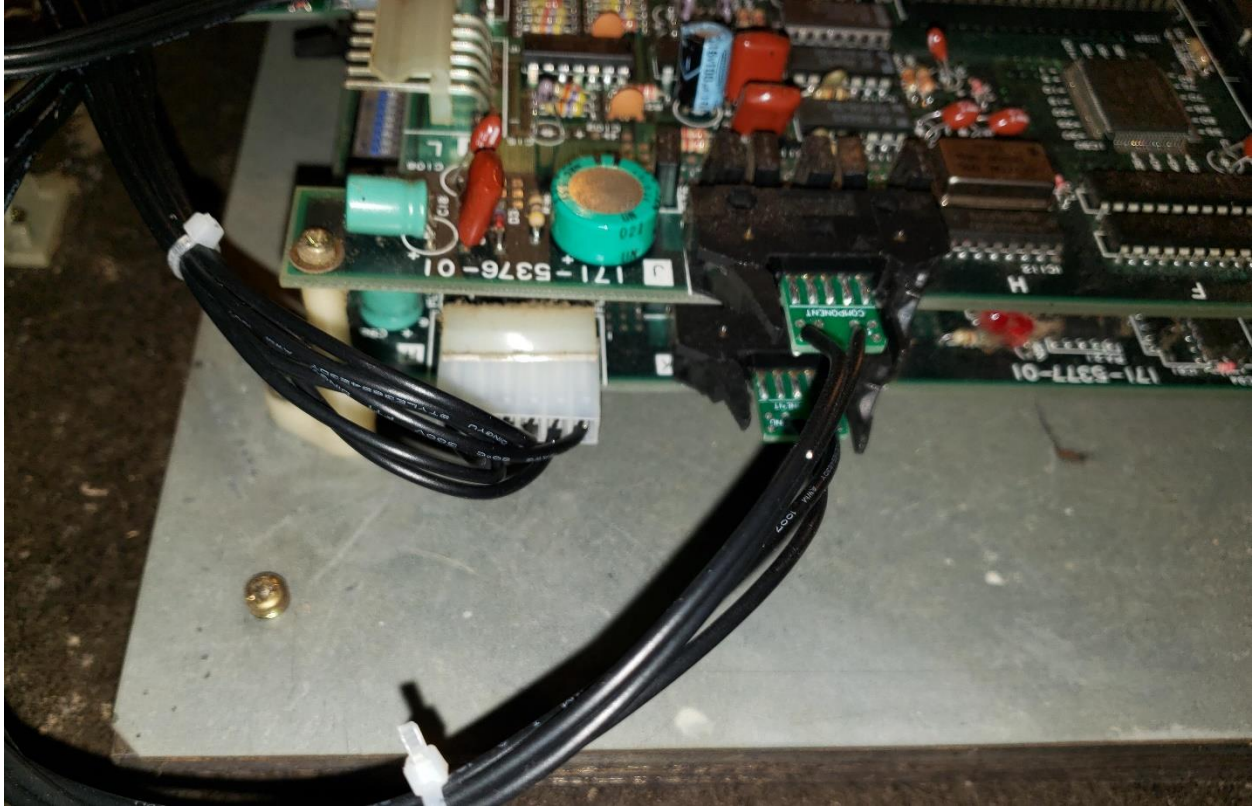
FIGURE 6. GAMEBOARD INTERFACE. VIDEO AND 5V POWER CONNECTORS
