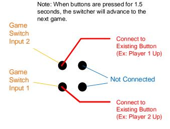
Game Switch Inputs Connected to Existing Control Panel Buttons
