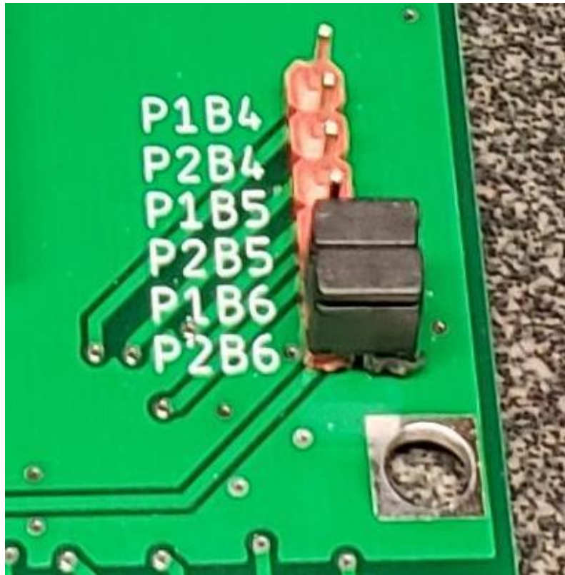
Figure 5. JAMMA Pins “27” and “e”, shown with both jumpers in place.
